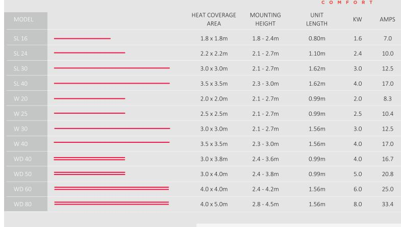
STEP 1 Determine the approximate measurements and the mounting heights of the area you want to heat.
