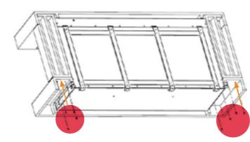
18) Using the suite screws, screw up through the bottom of the suite, through the suite fixing brackets and into the legs of the top section.
