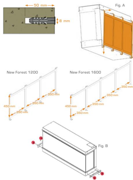
Before Installing the appliance onto the wall with the suite, secure the side-trims each side of the appliance as described in section 8.1 Preparing the Appliance.
