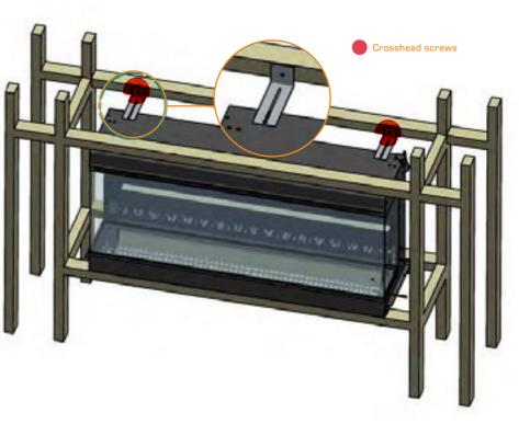
$\textbf{Step 4} - \textbf{Add finishing boards.} \ ^* \textbf{Important} - \textbf{fire must be in place before this stage*}$
