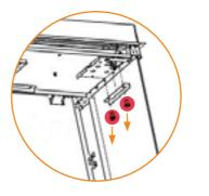
5) Carefully remove the side glass panels from each side, lifting from the bottom, inwards 75 mm then down to release then place both pieces of glass safely to one side.
