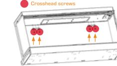
12) Remove the two highlighted screws that are located to the left and the right side of the gap and remove them using a crossheaded screw driver, offer the cover plate into position, lining the holes up, then screw the 2x screw back into position, securing the cover plate in place.
