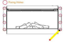
Remove the appliance from position and drill the appropriate drill size in the eight marked positions, to the correct depth.
