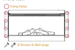
Once aligned screw the appropriate wall fixing screws into position, securing the appliance into place.
