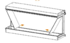
6) Unscrew the clamps on each side at the rear top of the appliance to release the rear glass.
