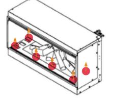
4) Unscrew the top clamps from each side of the side glass.
